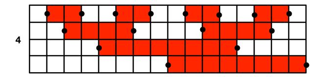
This algorithm is counting in a special binary code called Gray Code. The number gives the number of bits and each column is a binary number, with white meaning 0 and red meaning 1. The first column represents 0000 and one position after the last it has cycled back to 0000.
