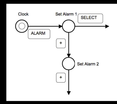
Working out the finite state machine of an alarm clock
