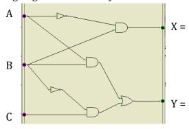
2. Complete the following truth table for output Y of the above circuit.
